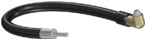
Designed with a heavy-duty flexible casing and core assembly for longevity. Fits any air or electric drill. Accepts 1/4" x 28 threaded drill bits and other accessories for close quarter drilling. Dimensions are 30" snake length, 1-1/4" head height, and 3/8" side to center. Drill capacity is 1/4".
