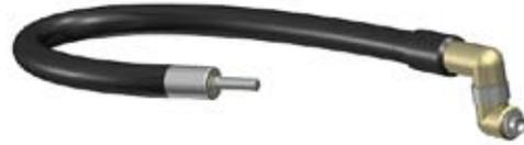
Ideal for drilling in areas inaccessible to regular 90° angle tools. Made of heavy-duty flexible casing and core assembly. Swivels 360° and can be locked into eight different positions. Accepts 1/4" x 28 threaded drill bits and accessories for close quarter drilling. Dimensions are 30" snake length, 1-1/4" head height 1-7/16" offset distance, 3/8" side to center. Drill capacity is 1/4".
