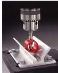
Drilling through the center of round stock can be a daunting task without the right tool. Center-It makes easy work of it by securely holding the stock in its vee cradle to stop the tube from rolling or slipping as you drill. It's 4"W x 5"L, and extruded from 6065-T3 Aluminum for years of use.
