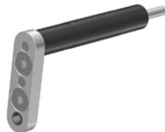
One of a kind drill attachment. Designed with a head thickness of only 7/16" for drilling in areas as close as 1". Fits any air or electric drill. Accepts 1/4 x 28 threaded drill bits and accessories for close quarter drilling. Dimensions are 6-5/8" long, 7/16" head thickness, 2-5/16" offset distance, 7/16" side to center. Drill capacity is 1/4".
