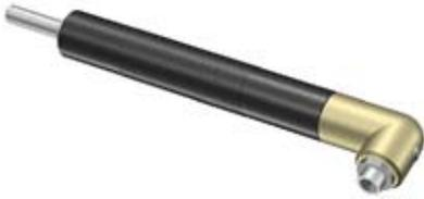
Heavy-duty economical drill attachment. Has 1/4" x 28 internal thread for use with standard threaded drill bits or miniature chucks. Fits onto any air or electric drill. Dimensions are 6" long, 1" head height, and 3/8" side to center. 1/4" capacity.
